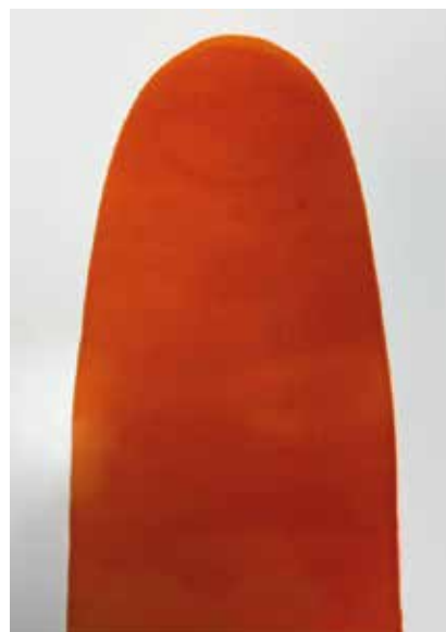
6mL Drawdown of Shade Coating tinted with 2% ColourFal® Zero 800-050 TRR Red Trans Oxide
